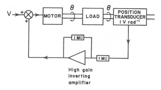
Derive an expression for the transfer function,  $\theta(s)/V(s)$  of the system with the feedback shown, where s is the complex frequency.
